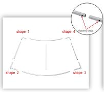
Connect corner sections to straight sections with matching shape codes.
